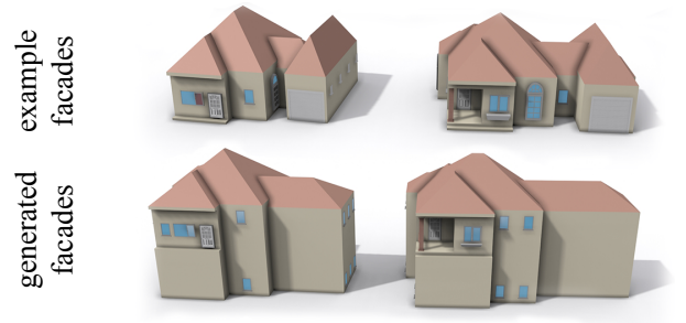
Figure 17: Results of applying an operations tree learned from unrepresentative examples: The operations tree for a family house was learned on single-story buildings (top row). When applied to two-story buildings, there is ambiguity that results in unexpected element placements (bottom row). Providing additional examples on two-story buildings would help to resolve the ambiguity.
